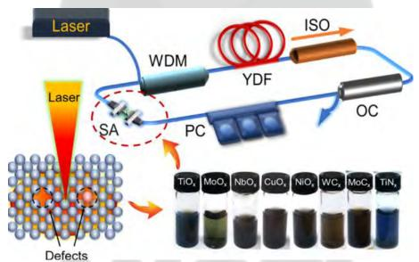
Figure 1 A universal nonequilibrium approach for the fabrication of plasmonic NCs along with simultaneous defect generation by fs laser processing in solution.
