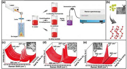
Figure 1. (a) Schematic of the formation and in-situ monitoring the Se colloids in various solvents. (b) phase transition of Se colloids. The in-situ monitoring results of Se colloids phase transition: (c) In dimethyl formamide, (d) In acetone, (e) In ethyl acetate.
