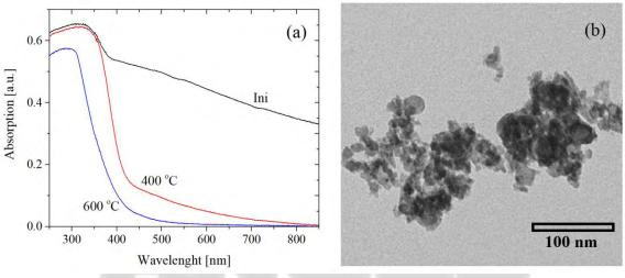
Figure 1 UV-Vis absorption (a) and TEM images of nanopowders BSO.
