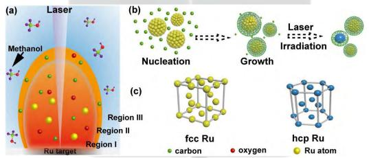
Figure 1 Illustration of the Formation of the Final Products in Methanol. (a) The state of the plasma plume in solution. (b) Nucleation and growth of crystals in Region II. (c) The crystal structure of Ru NPs.
