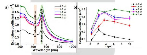
Figure 1 (a) Extinction coefficient for gold colloid nanoparticles produced by method of laser ablation at different pulse energy (pulse duration: 6.2 ps) (b) dependence extinction coefficient on pulse duration (at the peak of plasmon resonance-530 nm)
