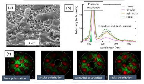
Figure 1. (a) SEM image of laser-fabricated nanospikes on a 1-µm thick gold film; (b) photoluminescence spectra of bacteria on Au nanospikes, acquired at different polarization; (c) microphotographs of the dead (red) bacteria, illuminated with 515-nm laser radiation with the corresponding polarization.
