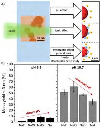
Figure 1 : A) Illustration of the fragmentation process, including visualisation of studied chemical influence factores [3]. B) Mass yield of particles after LFL using a 9 ns laser ( $532 \text{ nm}, 0.1 \text{ kHz}, 1.6 \text{ J/cm}^2$ ) [3].
