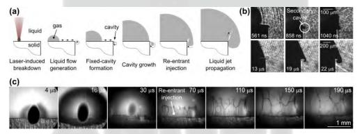
Figure 1. (a) Cavitation bubble development following laser-induced breakdown near a sharp geometry. (b) Formation of a fixed-type secondary cavity behind the edge. (c) Re-entrant liquid injection into the cavitation bubble.
