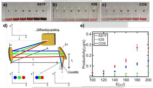
Figure 1. Image of the generated colloids as a function of the pulse energy I=100 µJ, II=120 µJ, III=140 µJ, IV=160 µJ, V=180 µJ, VI=200 µJ, for (a) SSTF, (b) IOS and (c) COS systems. (d) Implemented experimental setup of the SSTF technique for femtosecond laser ablation in liquid. (e) Productivity values obtained from the (a), (b) and (c) colloids proving the enhanced SSTF production.
