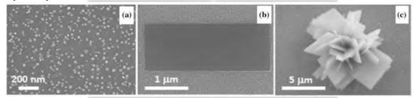
Figure 1 SEM images of typical nanostructures: (a) nanoparticles, (b) a nanoflake, and (c) a nanoflower obtained at the surface of ITO covered glass as a result of laser-induced deposition from solutions of supramolecular complexes [1].
