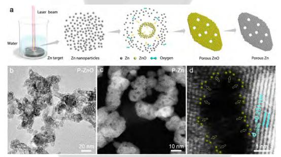
Figure 1. The preparation of P-Zn via PLAL. (a) Schematic illustration of the synthesis of P-Zn by laser ablation in O<sub>2</sub>-saturated water and the subsequent electroreduction. (b) TEM image of P-ZnO. (c) HAADF-STEM and (d) high-resolution HAADF-STEM images of P-Zn, the yellow dots mark the atoms around corners.
