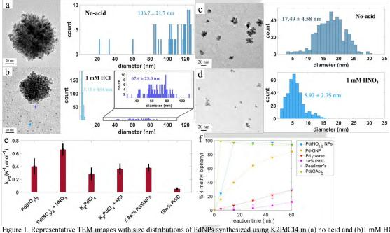
Figure 1. Representative TEM images with size distributions of PdNPs synthesized using K2PdCl4 in (a) no acid and (b)1 mM HCl, and Pd(NO3)2 in (c) no acid and (d) 1 mM HNO3. (e) kPd values for laser–PdNPs and other Pd-based catalysts. (f) 4-methyl biphenyl formation over time in the presence of Pd catalysts.
