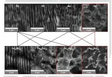
Figure 1 Scanning electron microscopy images of laser-ablated elemental metals and their alloys (50:50 composition) in water. Red frames mark metals that didn't form LIPSS while black frames mark the materials that formed LIPSS at the fixed laser parameters.
