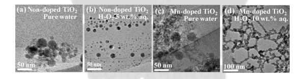
Figure 1 TEM images of  $TiO_2$  nanoparticles synthesized by laser ablation in pure water and  $H_2O_2$  aqueous solutions: (a), (b) non-doped  $TiO_2$ , (c), (d) 0.1 mol% Mn-doped  $TiO_2$ .
