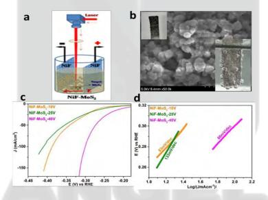
Figure 1. (a) Schematic illustration for the synthesis of NMs by EF-LAL, (b) SEM image (inset. Synthesized NPs on NiF and bubble formation during HER measurement, (c) HER polarization curve and (d) Tafel slope of synthesised NPs.
