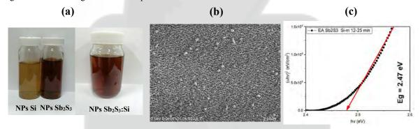
Figure 1 (a) Nanocolloids of Sb<sub>2</sub>S<sub>3</sub> and mono-Si by PLAL and their mix (b) Micrography of Sb<sub>2</sub>S<sub>3</sub> with mono-Si (c) Band gap Sb<sub>2</sub>S<sub>3</sub> with m-Si.
