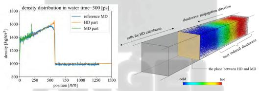
Figure 1. (a) Density distribution predicted for 300 ps after laser irradiation of a Ag target by a 10 ps laser pule by a hybrid MD-HD simulation (orange and green curves) and a pure MD simulation with longer computational cell (blue curve). (b) Snapshot of an interfacial region between MD and HD parts of the model shown for a time before the shock wave reached the interface. The atoms in the MD region are colored by temperature and the orange plane is the boundary of MD domain.
