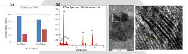
Figure 1. (a) Difference of the yield concentration in ppm of selenium present in MoSe<sub>2</sub> nanosheets synthesized in deep eutectic solvent (DES) and H<sub>2</sub>O. (b) EDS analysis of MoSe<sub>2</sub> nanosheets synthesized in DES showing a low oxygen existence, compared to the selenium peaks. (c) TEM image of MoSe<sub>2</sub>.Insert shows fringes indicating crystallinity.
