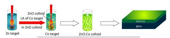
Figure 1 Schematic illustration of the experimental procedure used for preparation of cobalt-doped zinc oxide nanostructures
