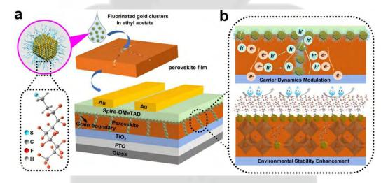
Figure 1 Laser manufactured hydrophobic Nano-Colloids as bifunctional interfacial mediator. a) Schematic illustration of interfacial embedding Nano-Colloids in the layer of perovskite. b) Schematic illustration of the function of Nano-Colloids for carrier dynamics modulation and improving environmental stability.
