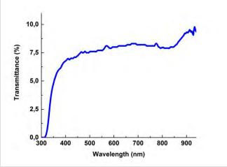
Figure 1 Transmittance of gold nanoparticles in solid sodium nitrate.
