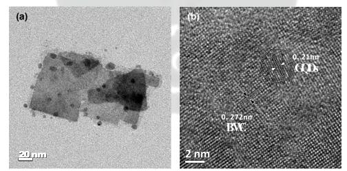
TEM images of ultrathin GQD-BWO nanosheets: (a) ultrathin GQD-modified Bi<sub>2</sub>WO<sub>6</sub> nanosheets (b) corresponding HRTEM detection of the GQD-modified Bi<sub>2</sub>WO<sub>6</sub> crystallographic plane.
