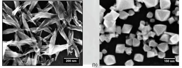
Figure 1 Single crystalline non-spherical metal oxide nanoparticles: (a) CuO nano-spindles, (b) PbO nano-octahedrons.
