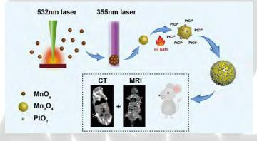
Figure 1. Schematic of formation of Mn<sub>3</sub>O<sub>4</sub>/PtO<sub>2</sub> nanocomposite and its application.
