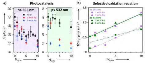
Figure 1: Effect of PuDEL of P25-TiO<sub>2</sub> (without and loaded with 1 wt% and 3 wt% of laser-generated Au NPs) on the catalytic activity shown for a): Photocurrent density *j* in photocatalysis<sup>[2,6]</sup> and b): Turn-over number (TON<sub>s</sub>) of ethanol to acetic acid during selective oxidation reaction<sup>[2]</sup>. Data are shown with respect to the number (N<sub>eyele</sub>) of laser irradiation cycles (~number of laser pulses) applied. Figure was taken from Ref. [2].
