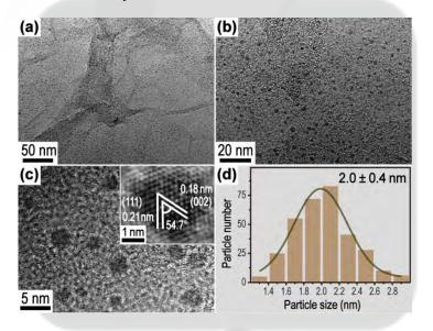
Figure. (a, b, c) TEM images of Cu/rGO NCs. (d) size distribution histogram of Cu NPs.
