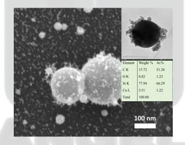
Figure 1 SEM image of Cu nanoparticles; insets: TEM image and EDX analysis
