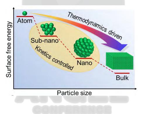
Figure 1. Kinetics dominated evolution of metal particles under pulsed high-temperature.
