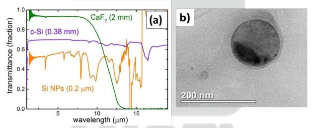
Figure 1 Near-mid IR optical properties of hyperdoped NPs: (a) transmittance spectra of fluorite substrate, c-Si wafer and S-hyperdoped Si-NP layer; (b) TEM image of silicon nanoparticles doped carbon and sulfur
