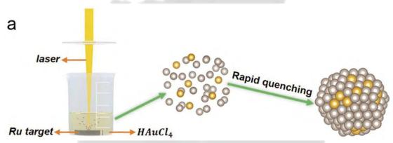
Figure 1 Schematic diagram of the synthetic process for single-atom catalysts.
