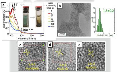
Figure 1 (a) Spectra of nickelocene during laser processing with photograph inset. (b) TEM image and size distributions of particles. (d, e, f) HRTEM images with lattice spacings of different particles observed in the same sample.
