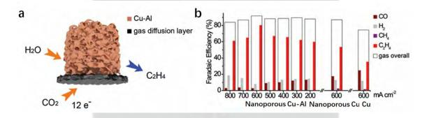
Figure 1. a. Schematic of electrochemical reduction of CO<sub>2</sub> to C<sub>2</sub>H<sub>4</sub> using the nanoporous Cu-Al catalyst on a gas diffusion electrode. (b) Electrochemical performance of CO<sub>2</sub> to C<sub>2</sub>H<sub>4</sub> with Cu-Al and Cu under different testing conditions.
