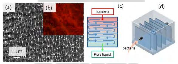
Figure 1. (a) SEM image of nanostructured Ti surface; (b) fluorescent photograph of the bacterial strains; (c) the upper view of flow-through filter and (d) its 3D model.
