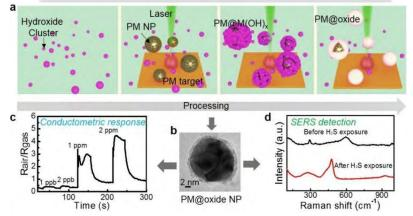
Figure 1 (a) The formation of the PM@oxide NPs, (b) a transmission electron microscopy image of a typical PM@oxide NP, (c) conductometric response of Au@SnO<sub>2</sub> NPs to H<sub>2</sub>S gas, and (d) SERS-based detection of H<sub>2</sub>S with Au@CuO NPs.
