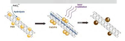
Fig. 1 Schematic illustration of the reduction of PdO to form Pd-PdO interface by laser irradiation.
