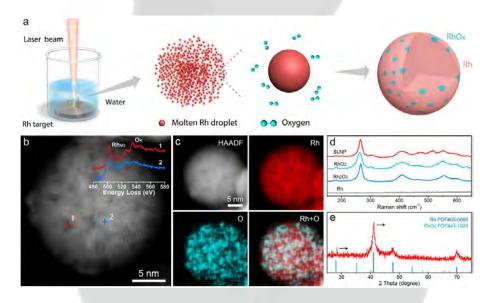
Figure 2. Preparation and Characterizations of SLNP catalyst. a) Schematic illustration on the PLAL synthesis and structure of SLNP catalyst. b) HAADF-STEM image of SLNP. The inset is the Rh M<sub>3</sub>-edge and O K-edge EELS spectra collected at point 1 and 2, respectively. c) EDS-mapping images of SLNP. d) Raman spectra of SLNP and RhO<sub>2</sub>, Rh<sub>2</sub>O<sub>3</sub> Rh references. e), XRD pattern of SLNP catalyst.
