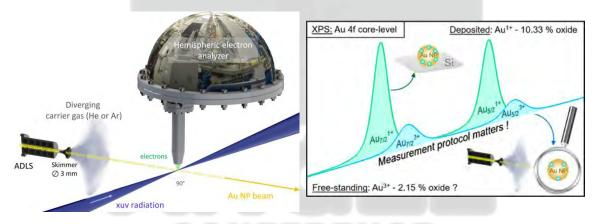
Figure 1 : (Left panel) Experimental setup of the XPS measurement of the Au NPs beam generated by means of the aerodynamics lens. (Right panel) Surface oxidation states of the Au NPs as a function of the measurement protocol.
