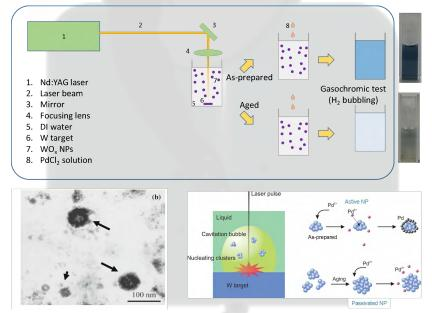
Figure 1 Laser assisted reduction process for synthesis of decorated LSPR materials WO<sub>x</sub>). TEM images of WO<sub>x</sub>@Pd (bottom left panel) core-shell structures. The other parts show the ability to detect hydrogen by these systems and the effect of resting time on core-shell structure formation.
