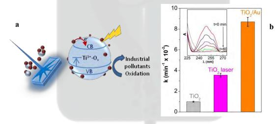
Figure 1 . a) Defects induced by laser irradiation on  $TiO_2$ ; b) kinetic constants of the photodegradation of the BTX/sulfolane aqueous solution, inset: UV-VIS spectra of the solution in presence of  $TiO_2$  laser treated catalyst.
