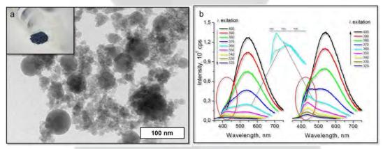
Figure 1 TEM image (a) and photoluminescence spectra (b) of TiO<sub>2</sub> powder.
