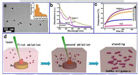
Figure 1 a. TEM images of Se@Au chain-oligomers colloid (Se@Au-1) and the bar graph of percent distributions of various oligomers. b. Optical absorption spectra of pure Se colloids that were ablated in water and aqueous NaCl solution, pure Au colloids (Au-1), and Se@Au-1. c. Temperature elevation of water and Se@Au-1 with increased power densities. d. A schematic of the formation processes of Se@Au
