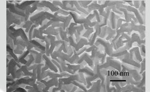
Fig. 1. NPs of Cu Pc at various stages of laser fragmentation after 10 min of fragmentation. Scale bar denotes 100 nm.
