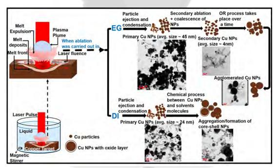
Figure 1 Schematic growth kinematics of Cu target ablated in EG and DI at a high laser fluence of 40 J/cm<sup>2</sup>.
