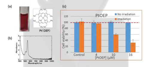
Figure 1 (a) photograph of the prepared Pt(OEP) nanoparrticle colloid and (b) its absorption spectrum. (c) Toxocity of Pt(OEP) nanoaprticles to rat PC12 cells, which were incubated in a culture medium containing the nanoparticles for 1 day, before(blue bars) and after (red bars) visible light (500-650 nm) irradiation.
