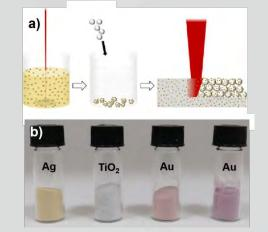
Figure 1. a) Scheme of the proposed methodology for laser generated nanoparticles supporting on polymer powders and the subsequent PBF-LB processing. b) Examples of a polymer powder after supporting of different laser generated nanoparticles.
