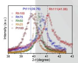
Figure 1 XRD profiles of NPs fabricated in RhPt mixed solutions.
