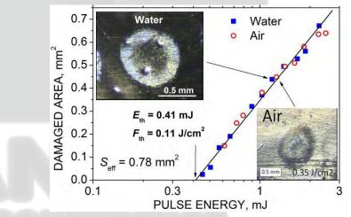
Figure 1 The area of the damage spots produced on the Sn surfaces in air and water as a function of laser pulse energy. The measured threshold energy, fluence and efficient spot area are indicated. The insets show optical microscope image of typical spots.
