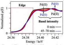
Figure 1 Time-resolved XANES spectra during laser irradiation with an interval of 5 min.
