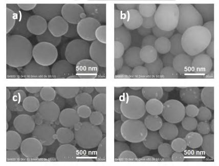
Figure 1 Images of nanoparticles and nanocomposites obtained by pulsed laser irradiation of α-Fe2O3 nanoparticles dispersed in different organic solvents: (a) toluene, (b) ethyl acetate, (c) acetone and (d) ethanol.
