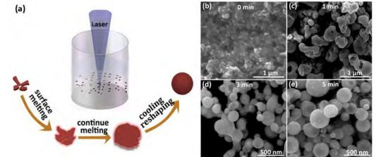
Figure 1 (a) Schematic illustration for the formation of the Cu nanospheres by laser irradiation. (b-e) The SEM images of the Cu nanoparticles with different laser irradiating time.
