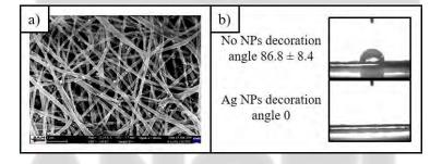
Figure 1 a) micrograph of the membrane decorated with the Ag NPs and b) contact angle test of the sample before and after the nanoparticle decoration, displaying that after the decoration, the membrane becomes hydrophilic.
