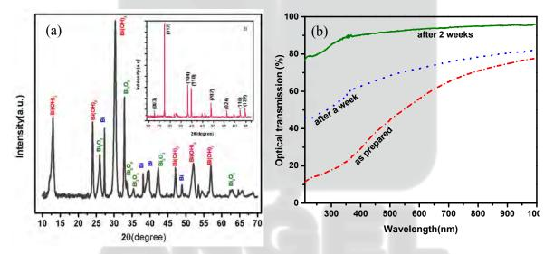
Figure 1 (a) XRD pattern of aged bismuth based nanoparticles that synthesized in water. Inset: XRD pattern of as-prepared nanoparticles in water (b) Optical transmission spectra of the bismuth based colloidal solution in water at different times
