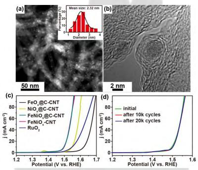
Figure 1. (a) HAADF-STEM image and (b) HRTEM image of FeNiO<sub>x</sub>@C-CNT, (c) the LSV curves of corrsponding catalysts with iR-compensation measured in 1 M KOH at a scan rate of 5 mV s<sup>-1</sup>, (d) LSV curves of FeNiO<sub>x</sub>@C-CNT before and after stability test.
