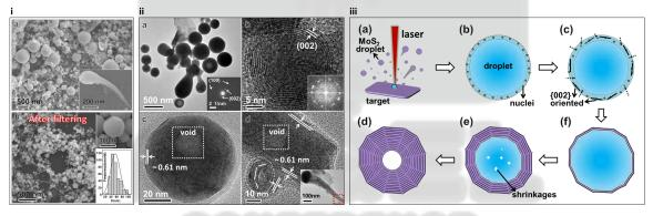
Figure 1 (i) Morphology, (ii) microstructure and (iii) growth mechanism of as-prepared MoS<sub>2</sub>.
