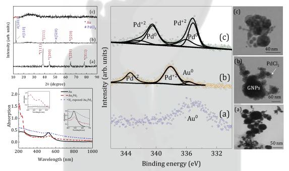
Figure 1 Left panel up: XRD, Left panel down: Absorption spectra of GNPs,Au<sub>1</sub>Pd<sub>2</sub> sample before and after hydrogen exposure, middle panel: XPS and right panel: TEM images of (a) GNPs, (b) Au<sub>1</sub>Pd<sub>2</sub> sample before and (c) after 10% H<sub>2</sub> exposure.
