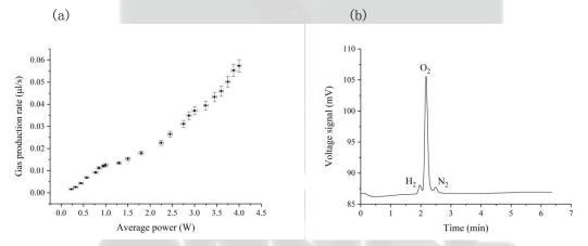
Figure 1 the relationship between gas productivity and average power as well as the gas chromatogram involved in this paper. (a) The relationship between gas productivity and average power. The laser amplifier used in the experiment is SOL ACE35F1KHp. The wavelength of the pulse laser is 800nm, the pulse width of the pulse laser is 35fs, the repetition frequency of the pulse laser is 1000Hz.
